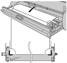
**5** While restraining the center of the roll media, turn the roll holder to take up any buckle in the media, pull the roll release lever toward you, then lock the paper guide.
